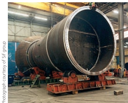
Figure 5.2 Wind turbine monopile foundation at Sif factory
