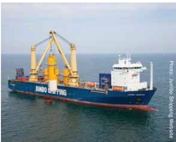
DP2 Heavy lift cargo vessel Jumbo Javelin
