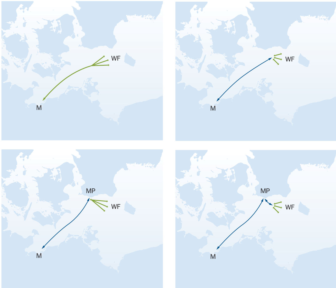
FIGURE 7.1 ALTERNATIVE APPROACHES TO WIND TURBINE INSTALLATION
